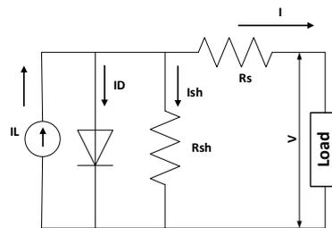
$$I = I_L - I_o \left[ \exp\left(\frac{V + I \cdot R_s}{a}\right) - 1 \right] - \frac{(V + I \cdot R_s)}{R_{sh}}$$
