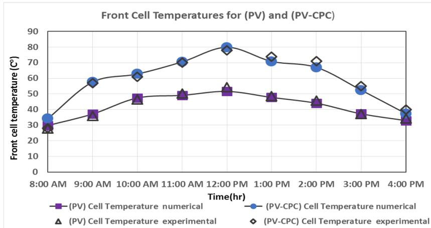
Figure 10: Comparison between numerical and experimental results of Front cell temperatures with and without concentration
