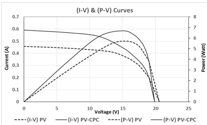
Figure 12: Comparison of (I-V) and (P-V) curves with and without concentration
