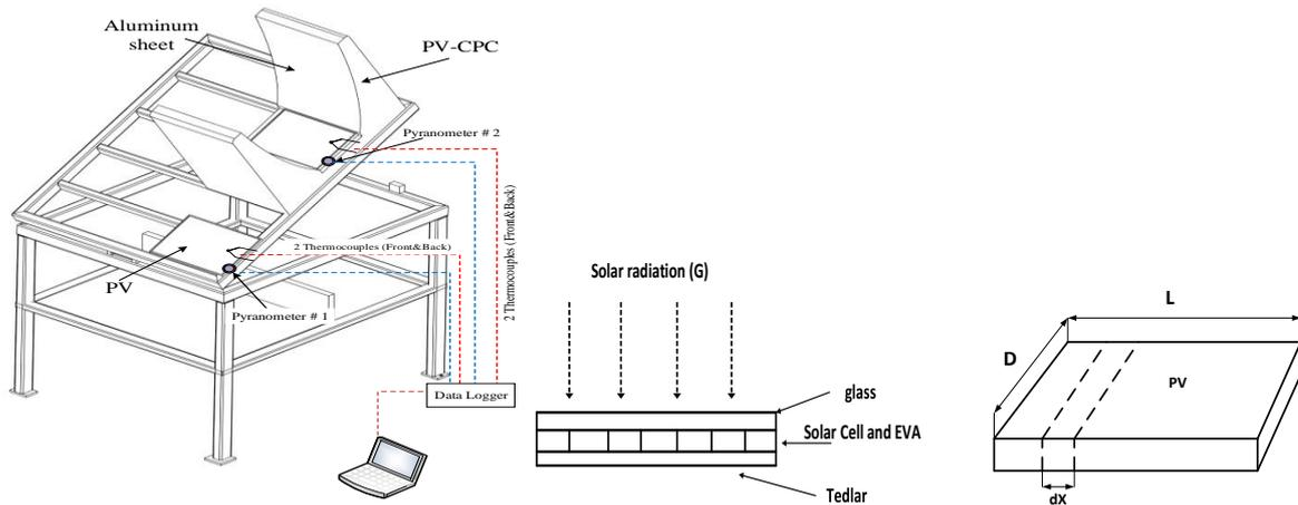
Figure 1: Schematic diagram and cross-sectional view of a (PV-CPC) collector
