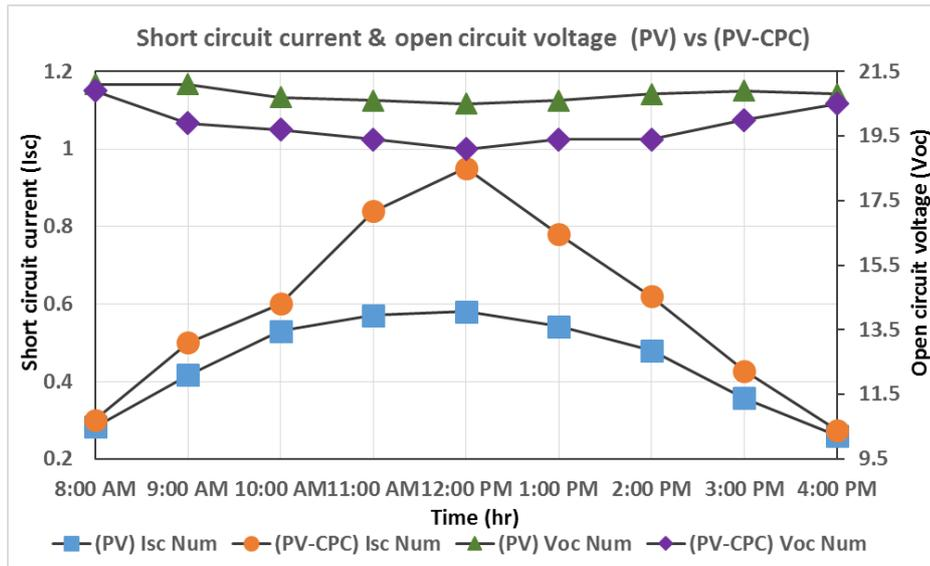
Figure 8: Variations of short circuit current and open circuit voltage for the two systems
