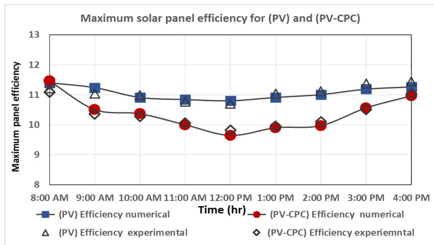
Figure 11: Comparison between numerical and experimental results of maximum output efficiency with and without concentration.
