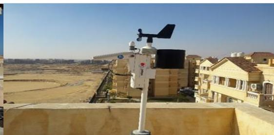
Figure 5: a photograph of the portable meteorological weather station
