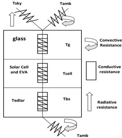
Figure 2: Thermal resistance circuit diagram for a PV-CPC collector
