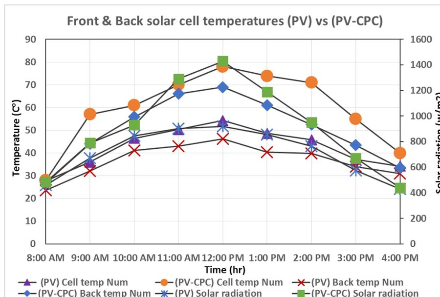
Figure 7: Variations of front and back solar cell temperatures for the two systems
