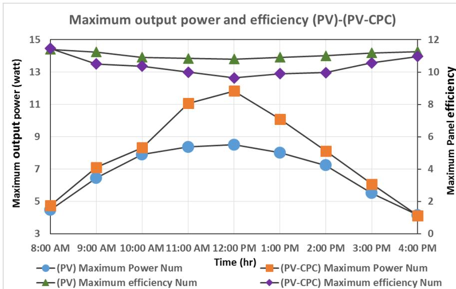
Figure 9: Variations of maximum power point and electrical efficiency for the two systems
